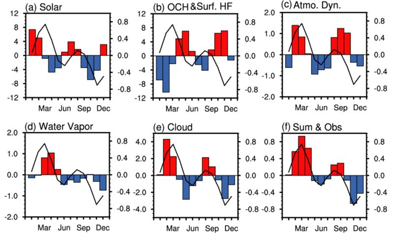
**Fig. 3** Annual cycle of partial temperature changes (K) of surface temperature average over (15°S-25°N, 105°-150°E) due to changes in (a) solar radiation at the TOA, (b) oceanic dynamic and ocean/land heat storage (OCH) and surface heat flux, (c) the atmospheric dynamics, (d) water vapor, (e) cloud, (f) sum of all individual feedback processes. The black solid lines in (a-f) refer to the observation (K).
