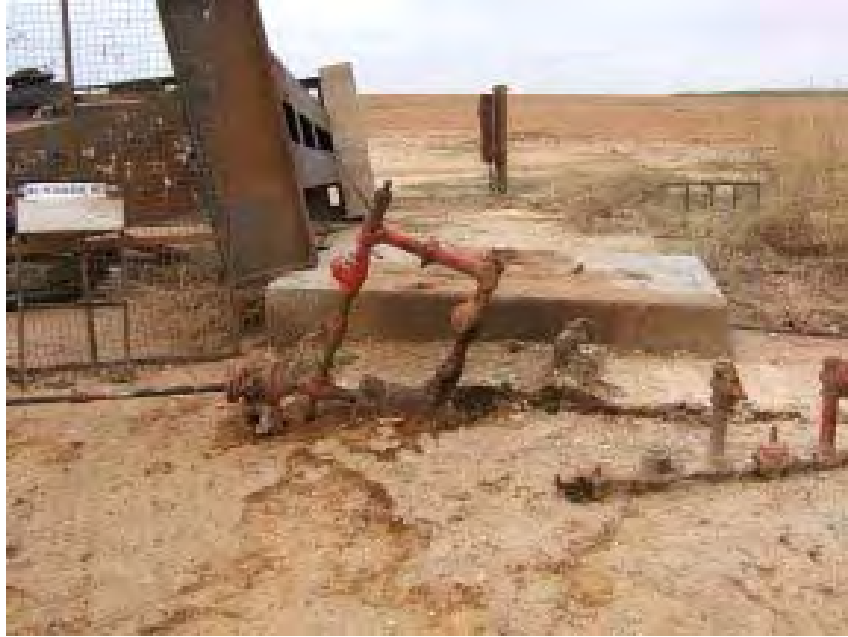
A pump jack was pulled out of the ground by a tornado in northwestern Martin County. Photo courtesy: Mark Cochran
