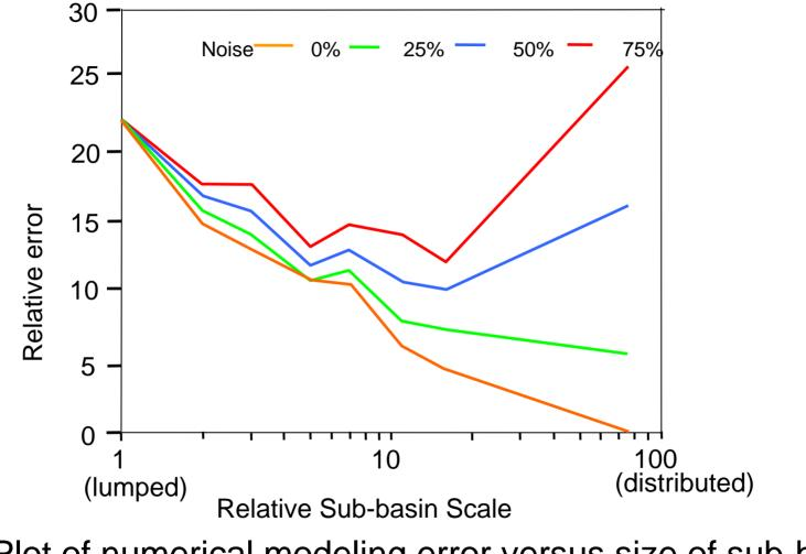
Plot of numerical modeling error versus size of sub-basin for various levels of radar data error (Koren et al. 2003)
