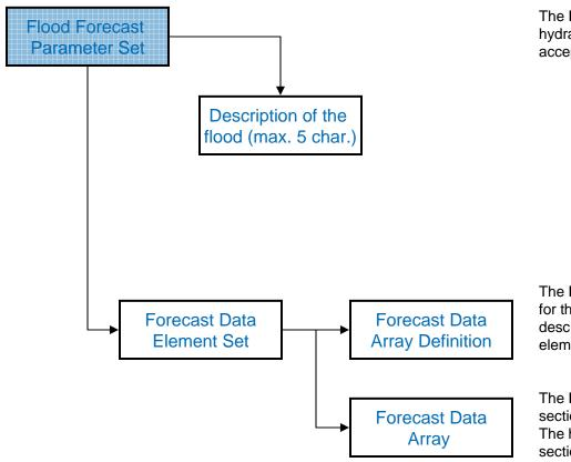
The **Flood Forecast Parameter Set** node specifies both the hydraulic forecast data and its metadata. This structure is able to accept multiple forecasts or time series if needed.
