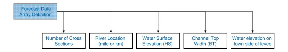
**Number of Cross Sections** defines the number of cross-sections used in the hydraulic flood model.
