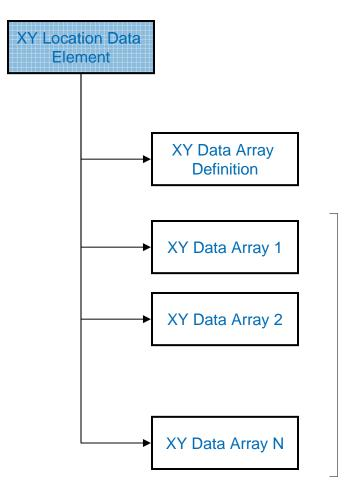
The **XY Data Array Definition** node stores the metadata for the entire collection of data arrays for multiple flood mapping scenarios. For every mapping scenario (represented by a **Data Array**), the node provides a name, description, data type, measurement units and location of the data element.
