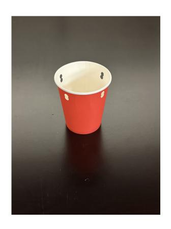
With the fifth cup, double punch holes on each side of the cup. This is because you'll need the holes to be a little bigger on the cup that goes in the middle of your anemometer.
