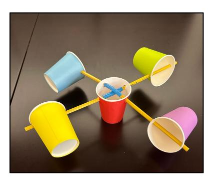
Attach the final cup to the anemometer. All of your cups should now face the same direction.
