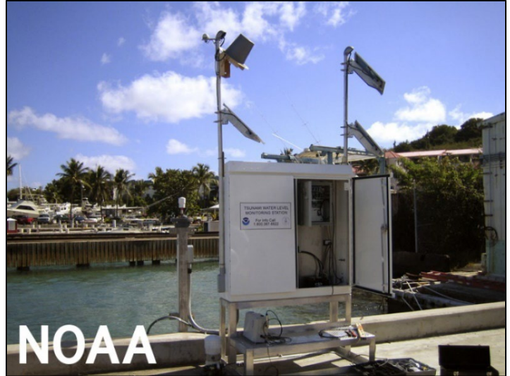
Observations from coastal water-level stations help the tsunami warning centers issue accurate tsunami alerts. (NOAA)
