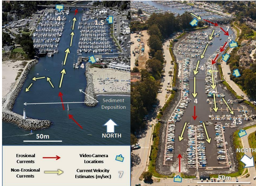
Figure 1: Location of strong and erosional currents inside Santa Cruz Harbor during the 2011 Japan tsunami (from Wilson et al., 2012).
