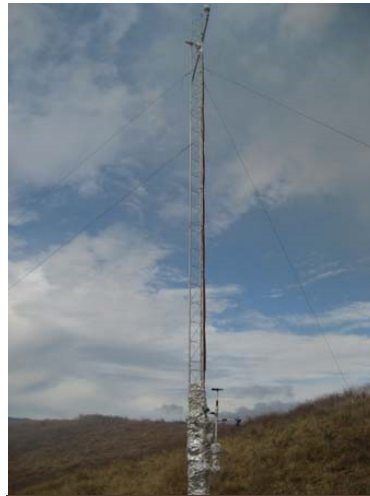
40 foot Weather Tower with several instruments on it
