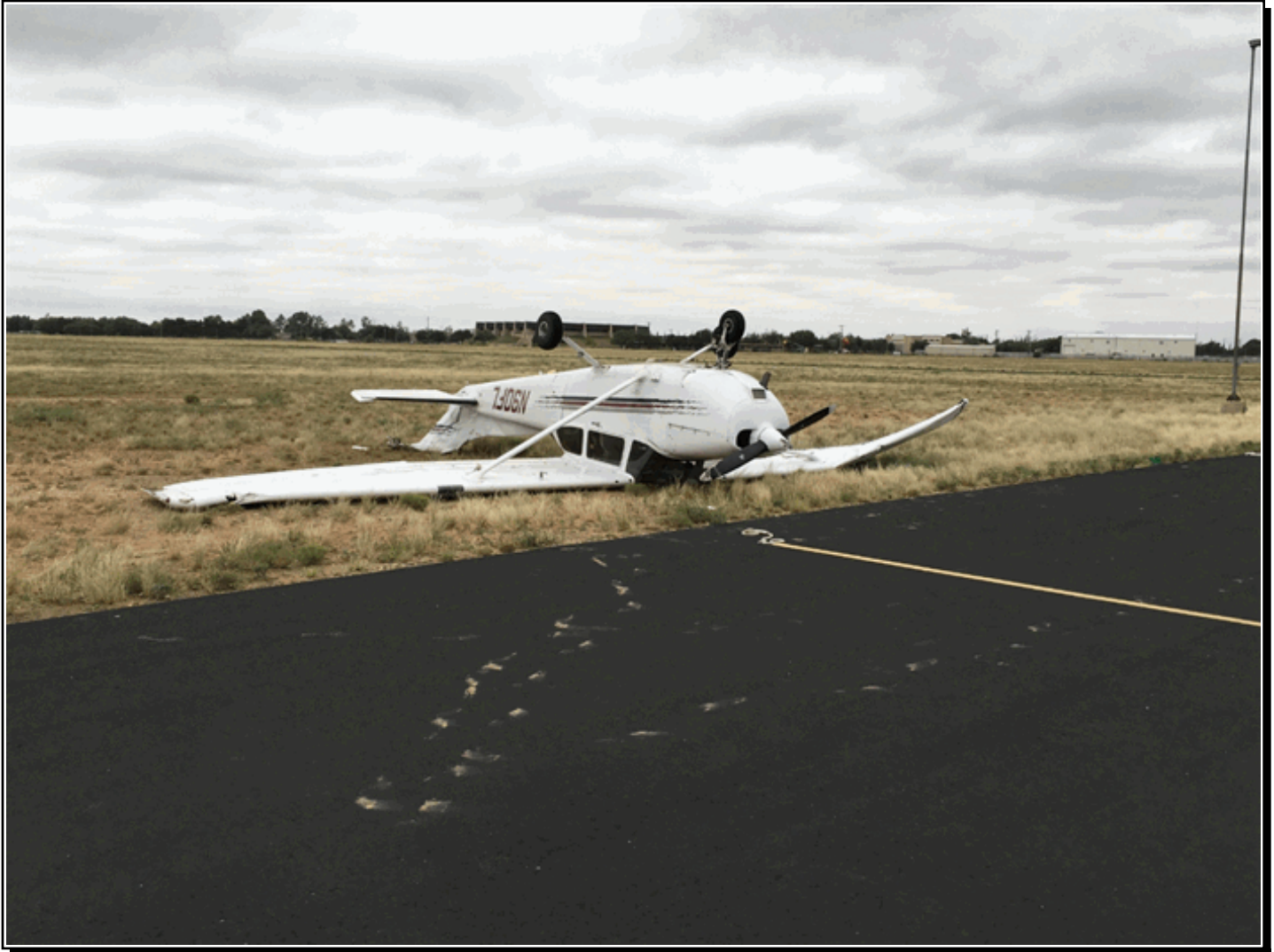
A single engine plane was ripped from its tie down and rolled an estimated 50 yards at the Midland Air Park in Midland, TX from thunderstorm winds. Photo is courtesy of the NWS survey team.
