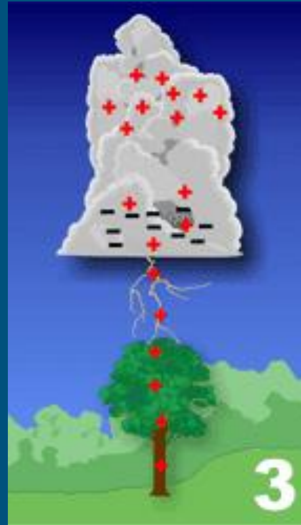
Return Streamer Connects, Visible Bolt
