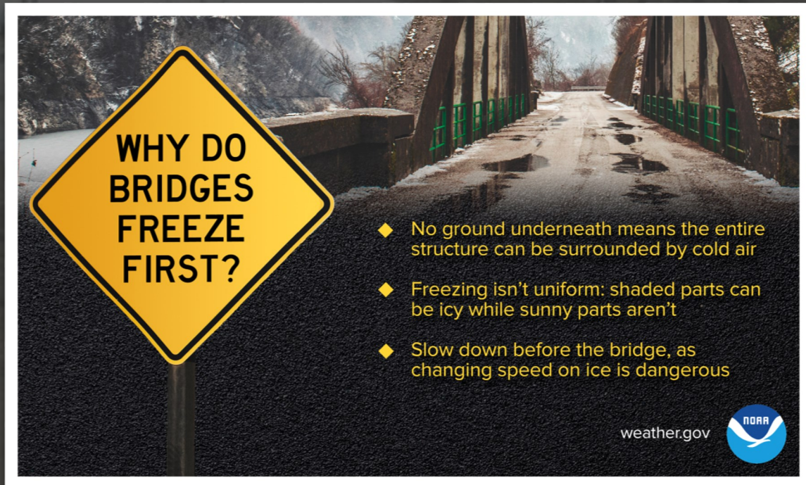
Figure 7: Infographic depicting reasons why bridges freeze particularly early on compared with other surfaces.
