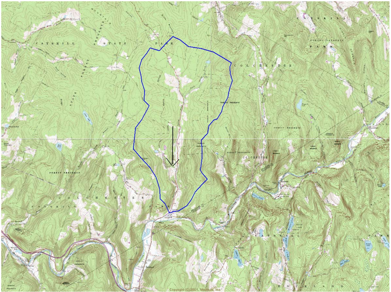
Figure 13a. Watershed boundary created from Maptech Terrain Navigator software of Spring Brook at landing strip. Arrow indicates direction of streamflow.
