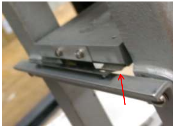
Figure D-3. Example of Bent Flexures
