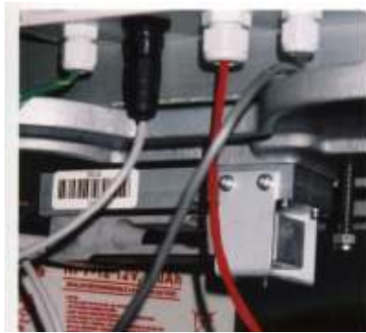
Figure 9.3 Load Cell Sensor (Sutron) with UPC
