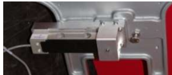
Figure 2.4. Load Cell Mounts Under Stage
