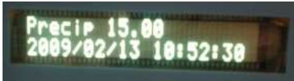
Figure 2.8. Precip Display Gives Bucket Level (15.00) and Current Date and Time
