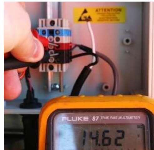
Figure 7.4 Battery Voltage for Logger (Red and Adjacent Black)
