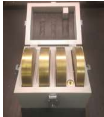
Figure 6.3 Select Three 4111G Brass Weights
