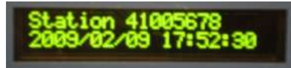
Figure 2.11. Station ID Number – Ensure it appears like this example SS00NNNN
