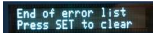
Figure 7.13 Use Down Arrow to Scroll and Search for Any Other Error Codes
