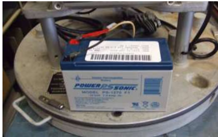
The red wire is the Positive Lead
