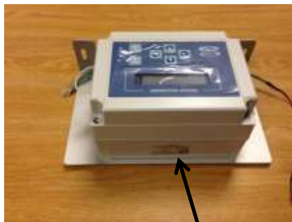
Figure 9.5 Precip Recorder has metallic decal on top side of box
