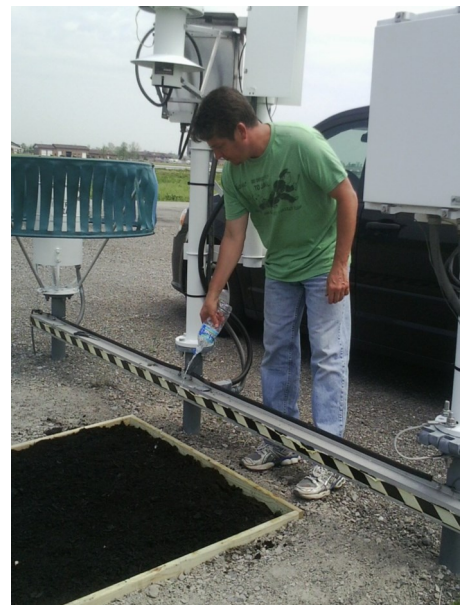
Tony Allen, Electronic Technician maintains a vegetation box that is needed under the temperature and dew point sensors.
