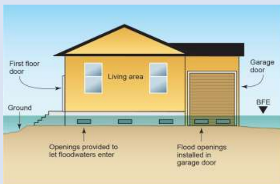
Figure 4a and 4b: Schematic example of wet floodproofing (4a, left) and dry floodproofing (4b, right).
