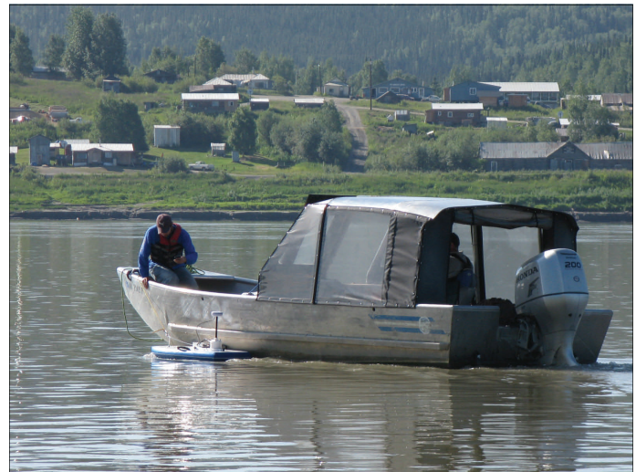
The SonTek M9 ADP (pictured above alongside boat) was used this summer to take flow measurements on the Koyukuk River at the villages of Allakaket, Bettles, Hughes, and Huslia, the Kobuk River at Kobuk, and on the Yukon River at Galena, Nulato, Ruby, and Tanana.
