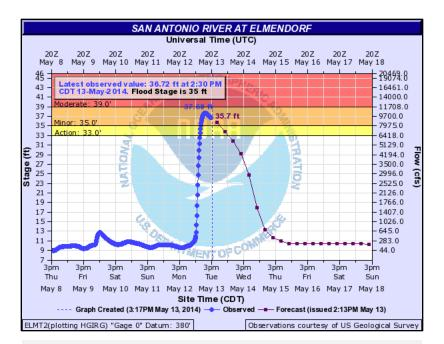
San Antonio River at Elmendorf Hydrograph. The river level increased quickly from 9 feet to 37 feet on the morning of Tuesday, May 13<sup>th</sup>. Action Stage is 33' and Minor Flood Stage is 35', so some minor flooding occurred. The river is expected to be back below flood stage by the morning of Wednesday, May 14<sup>th</sup>.
