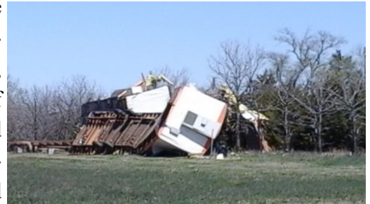
Unanchored mobile home rolled 25ft near northeast Wichita due to very strong straight-line damaging winds around midnight April 3rd. Photo courtesy of NWS Wichita.
